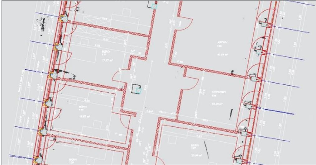
Differences between survey documentation with the aid of laser scanning and manual measurement.
