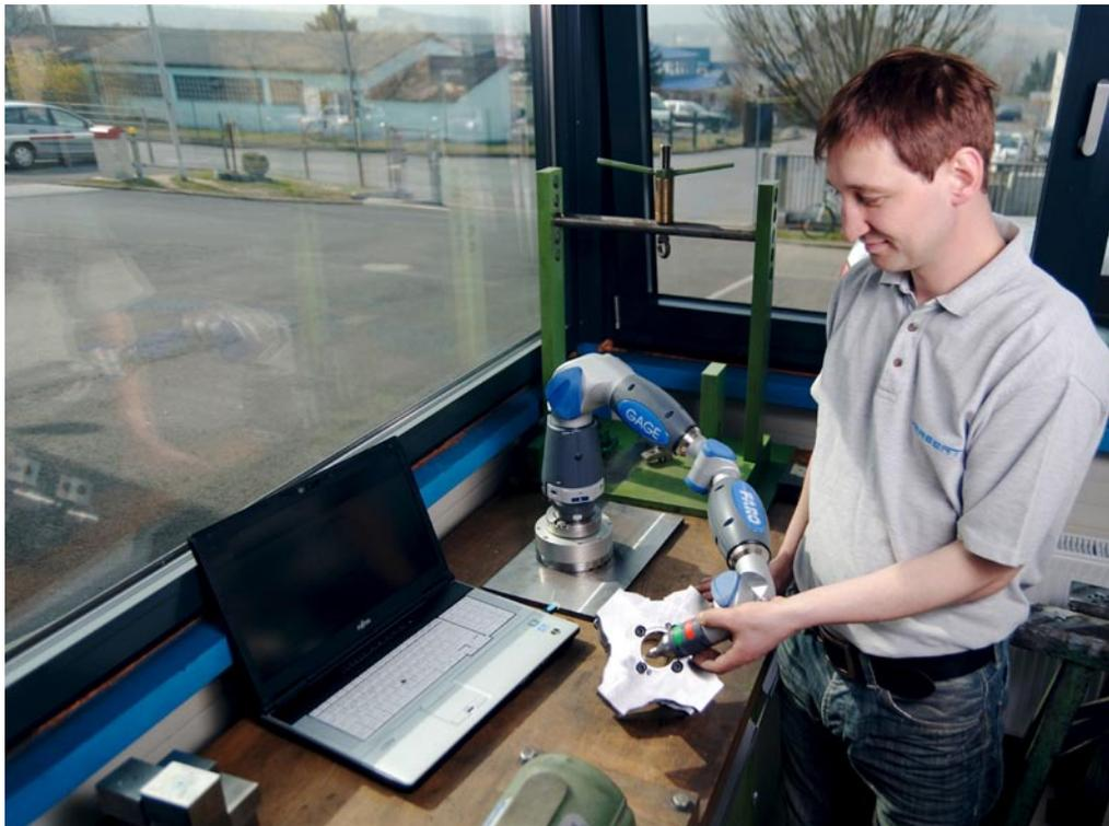
Use of the FARO Gage for interim checks during the production process.
