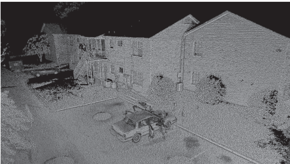
Figure 3. Point cloud data resulting from the 3D scan of the apartment complex.
