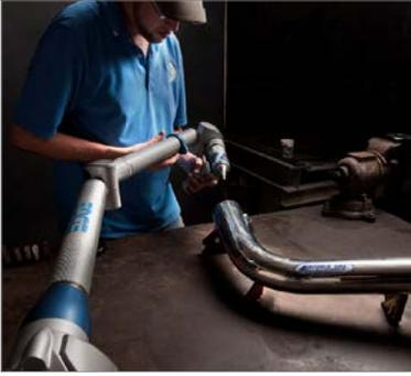
For areas that are difficult to capture accurately using the scanner, operators can alternate between the hard probe and the laser line probe within the same part. The data collected is automatically imported into the software, where it calculates deviations compared to master data and connects to and provides corrections to in-process CNC benders.
