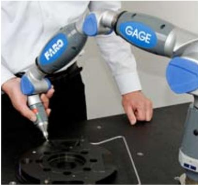
Portable CMM ball probes typically use grade 5 spheres. This means that the diameter of the ball is known to +/- 5.63 microns with a sphericity of +/-0.13 microns.<sup>4</sup> Some manufacturers are now measuring and stamping the diameter of the probe right on the ball probe itself, accurate to 1/10 of a micron. This further reduces the uncertainty in measurement results.
