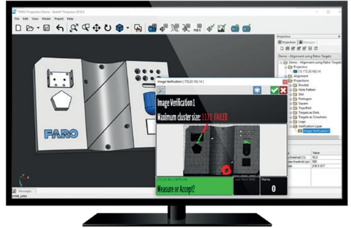
In-Process Verification (IPV) with FOD check
